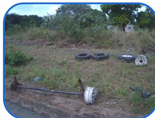
WHI's damaged water trailer (top); the trailer's damaged axle (above).
